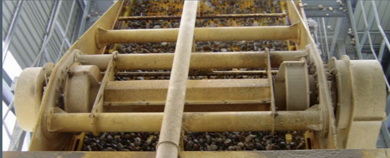
Otomatik yağlama sistemi Automatic lubrication system
