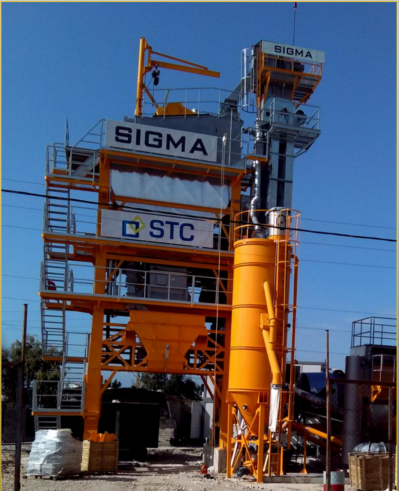
LEBANON/ BEIRUT YACOUB & ZIAD SHAHEEN COMPANY (S.T.C.) 120 T/H ASPHALT PLANT
